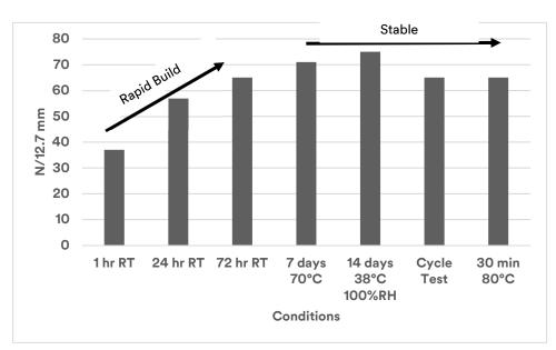
3M ST1200 Tape has excellent initial adhesion at assembly and outstanding long-term adhesion over all environmental conditions during vehicle life.
