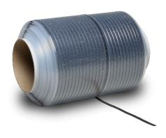
3M<sup>™</sup> Acrylic Plus Tape ST1200 is a 1.20 mm (0.047 in) thick, black acrylic foam tape, constructed with two different adhesives, used to attach weatherstrip and/or gasket seals for automotive and industrial applications.
