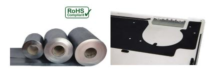
JONES 6-20-0137 heat spreading materials are natural graphite sheet with high thermal conductivity and high flexibility. It is manufactured entirely from natural graphite flakes with no fillers or binders. It possesses unique functions such as eliminating hot spots, shielding components and reducing skin temperature of electronic devices. It is an ideal heat spreader for thermal management in limited space.
