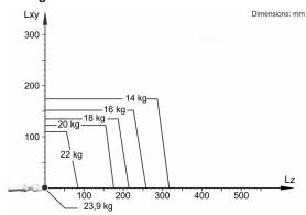
The KR 20 R1810 CR is designed for a rated payload of 20 kg in order to optimize the dynamic performance of the robot. The maximum payload of 23.9 kg applies only if the position of the center of mass is 0 mm and a supplementary load optimized for the load case is mounted. The specific load case must be verified using KUKA.Load or KUKA Compose. For further consultation, please contact KUKA Support.
