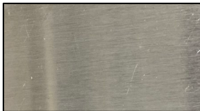
Test coupon after 10 sec. of cleaning by Flux-Off No Clean EXTRA
